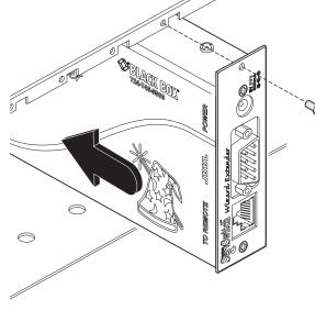
Mounting the REMOTE module using the single cut-out rack plates
